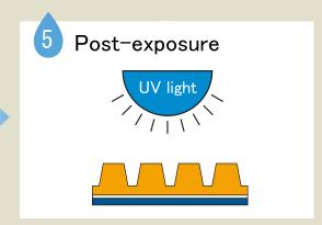
Expose the developed plate after drying again to UV light in order to get stability. Post exposure time.
