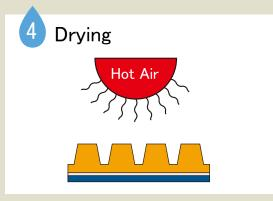
Dry the plate in hot-air dryer after taking-off the surface water with sponge roll.
