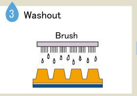
Washout exposed plate with water. Use the special washout machine suitable for TOYOBO PRINTIGHT®
