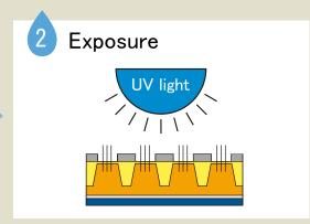
Expose plate to UV light having 360nm wave lengths.
