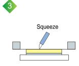
After spraying 20-30 seconds, wipe off the excess liquid carefully with a squeeze several times.
