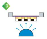
Contact a positive film onto the photo-sensitive plate and apply UV exposure or metal halide lamp.
