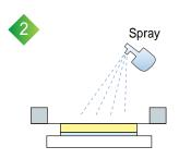
Place the frame with screen fabrics on the photo-polymer plate and spray water upon it thoroughly with a kind of sprayer.
