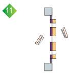
Washout unexposed polymer with tap water using soft brush or sponge.
