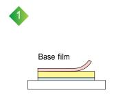
Peel off the base film and place the photo-polymer on the flat board made of foam polystyrene, ...etc.
