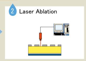
Depicted digital images through an IR laser head to the mask layer directly.
