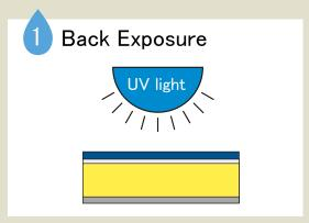
Expose UV light from the back side of COSMOLIGHT® to make floor first.
