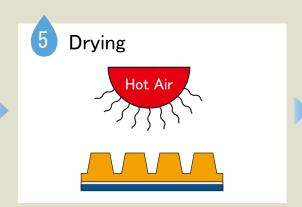
After wiping off the surface moisture by sponge roll, dry in hot air dryer.
