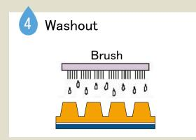
Washout the exposed plate with COSMOLIGHT® washout unit.
